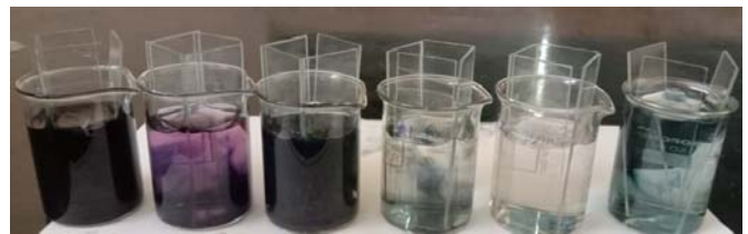
Figure 1. Changes in color observed while induction and deposition of Polyaniline thin films.
